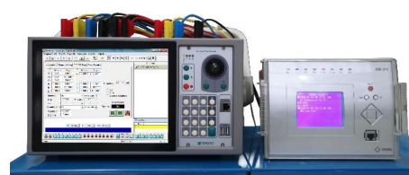
Local control with touch screen for relay testing
