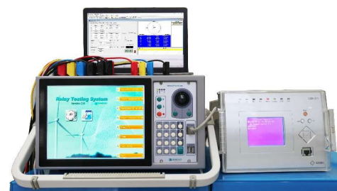
PC control for relay testing
